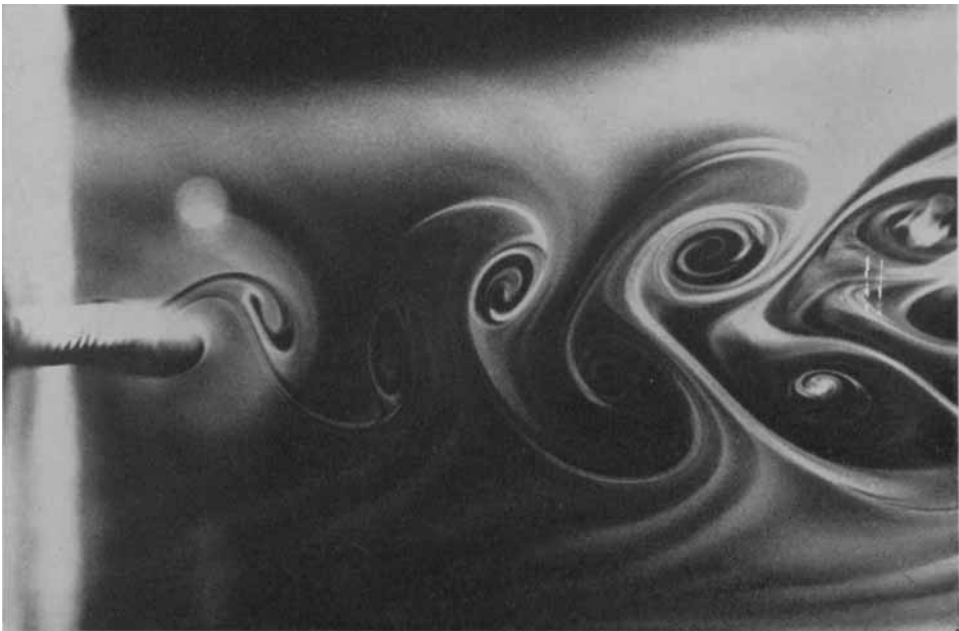
FIGURE 9. Vortex shedding from a stationary six-stranded cable at a Reynolds number of 220. Shedding frequency f_n = 41 Hz.
